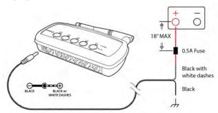
Connect the BLACK wire with WHITE dashes to +12V and the BLACK wire to chassis ground. Install the fuse no further than 18" from the battery.
